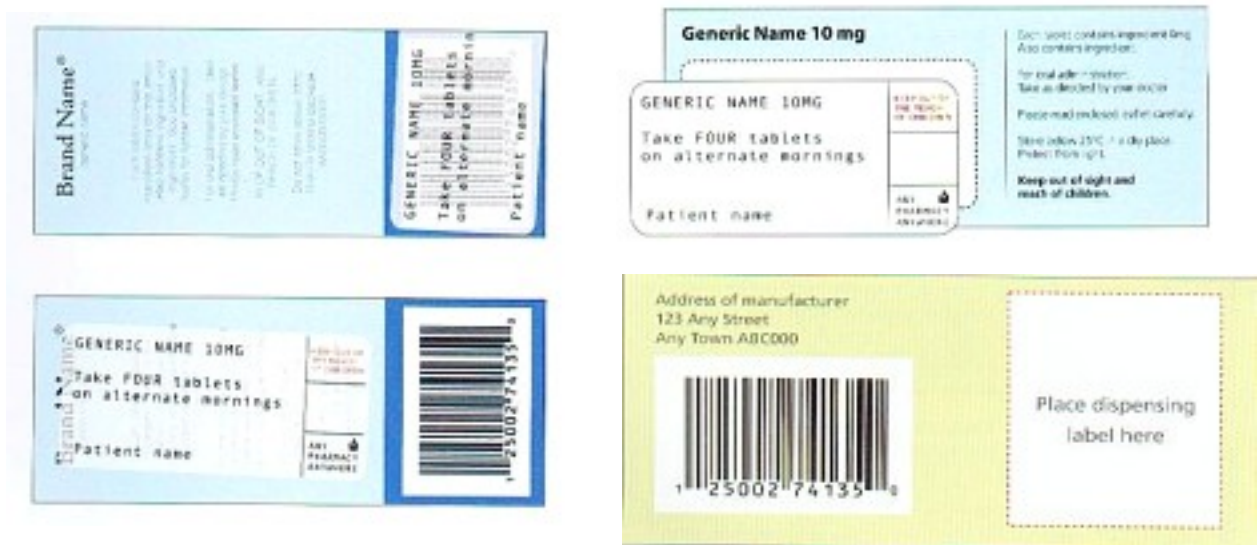
Figure 5: Secondary packaging should have a clearly marked space of at least 70 x 35 mm for the dispensing label 7
